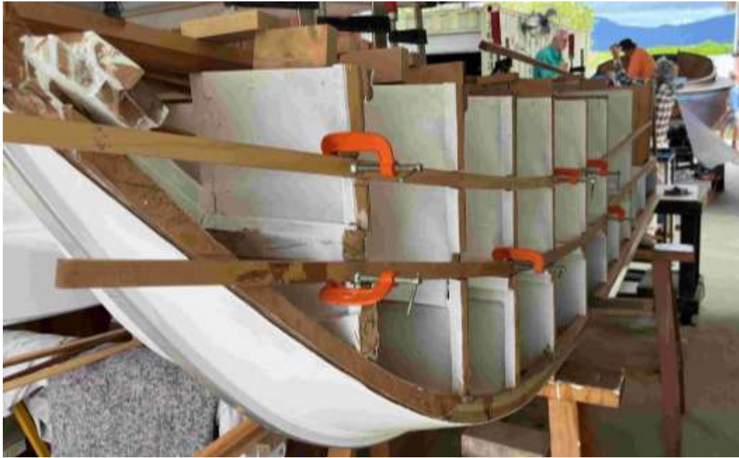
Port side waiting for the inner and outer gunwales to be fitted.
