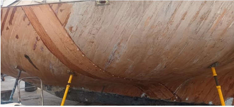
Second laminate of the double-diagonal layup commenced
