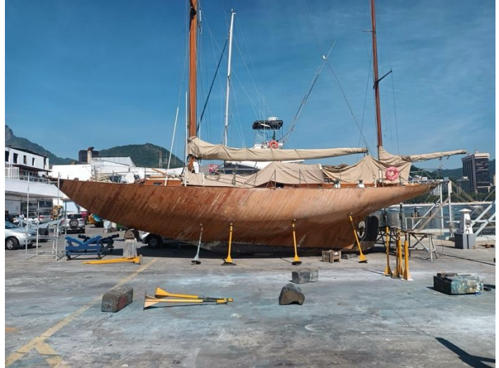
Double diagonal complete, fairing started.
