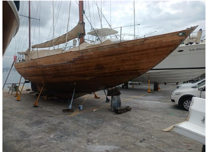
Sanding complete, revealing a midships repair..!
