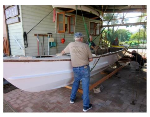
The 16'Skiff: Has been cleaned inside and out and has been flipped over. She will rest right-side up on BT's trailer for the foreseeable future, and will have her internals sealed with paint to prevent any further deterioration, then pest-proofed with fine birdwire.
