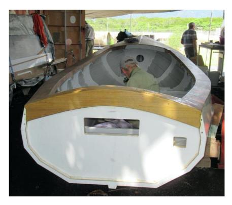
Roger's 15' strip planked canoe is hull-complete with some bracing ribs installed, and other ribs & seat frames being laminated. She will be a thing of beauty once completed – also this year! We have been busy!
