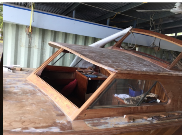
Windows removed and frames prepped.
