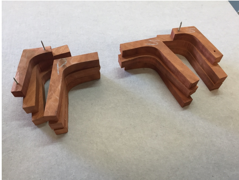
These are the corner inserts to join the side coamings to the front, layered in a brick pattern.
