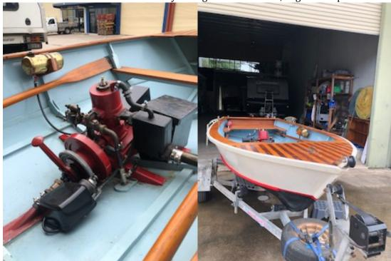
Cruises around 5 - 6 knots. Carby & magneto overhauled, engine in top nick.
