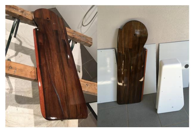
and the centerboard has also had it's lead insert installed. GRP sheathing to be wrapped in place very soon.
