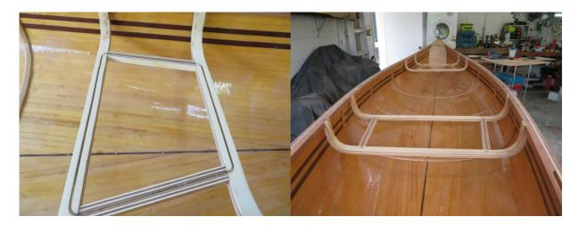
**Tom's Pathfinder:** Cockpit seating almost complete, centreboard about to be fitted, boomkin retainer made & fitted, upper deck painting complete, cockpit coaming to commence shortly, tabernacle support pillar made, to be fitted shortly.
